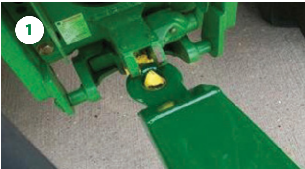
Check the condition of the towing eye for signs of wear or damage.
