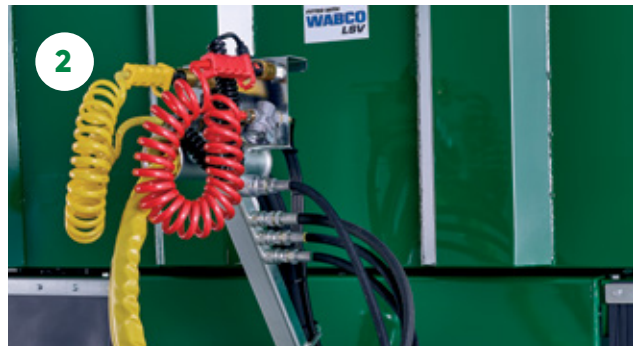
Check the condition of the air and hydraulic connections and hoses.
