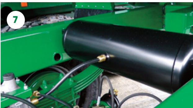
Drain water from air reservoir (where applicable).
