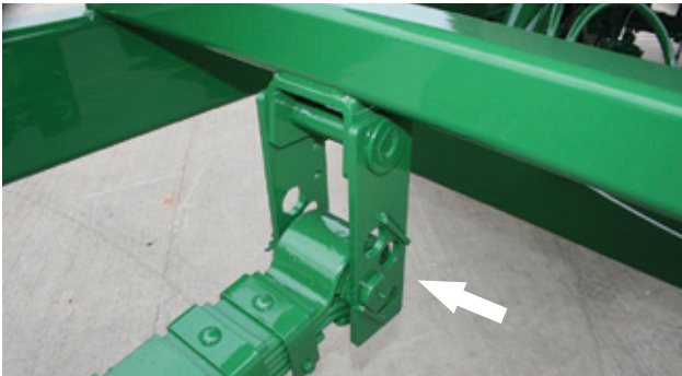
Grease the sprung drawbar pin (where applicable).
