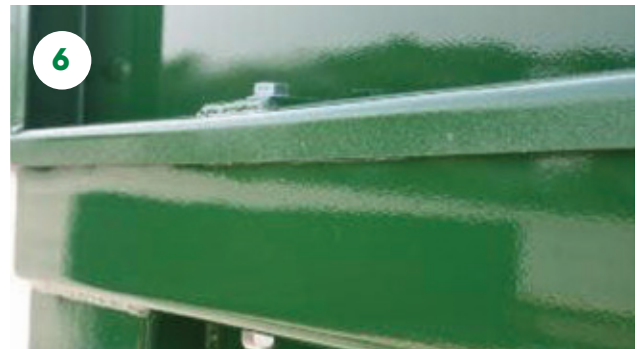
Check side extension bolt security.
