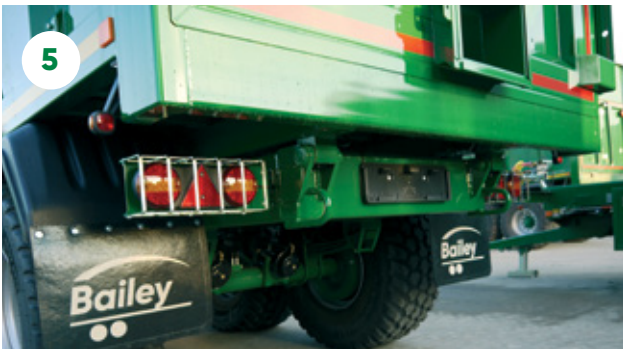
Check lights & reflectors for correct operation & damage.
