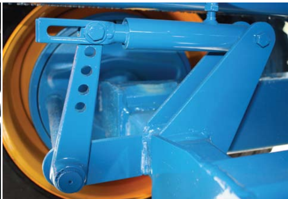
Splined brake lever arm: free-play adjustment requires removal from camshaft and replacement on alternative spline
