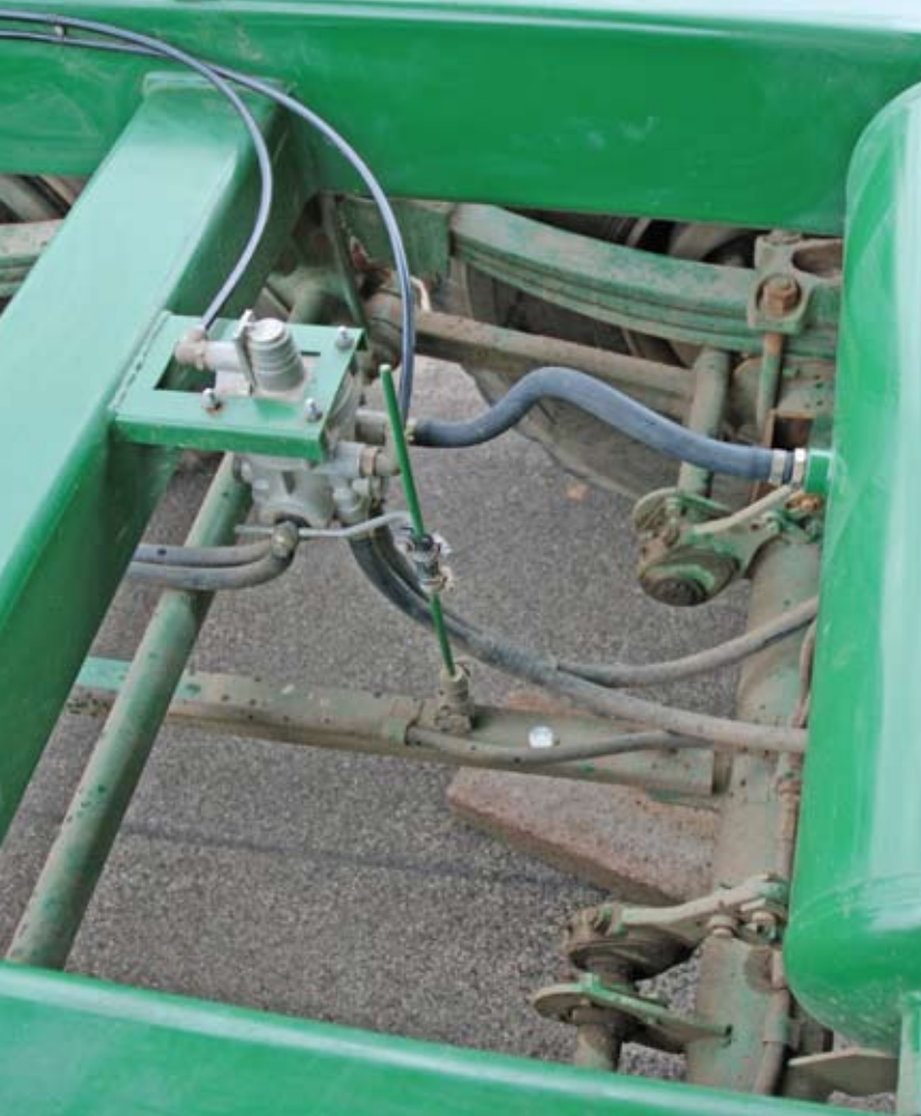
Pneumatic load sensing (Note: balance beam between axles and 'screw-type' slack adjusters)
