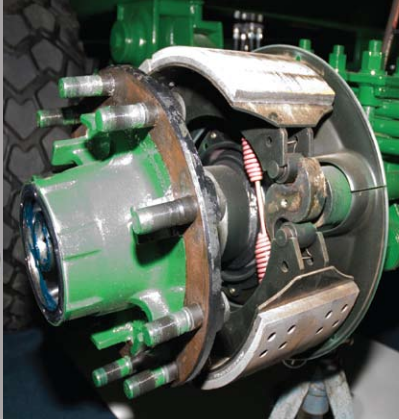
Ø420 x 180mm high-speed brake: Riveted shoe 'S' cam actuation
