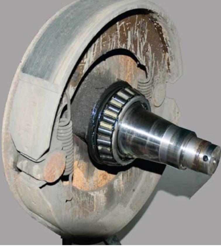
Ø400 x 80mm Ag. spec: Bonded shoe 'flat' cam actuation
